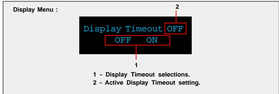
Use the “LEFT” and “RIGHT” buttons to highlight the desired option and select it by pressing the “ENTER” button.
