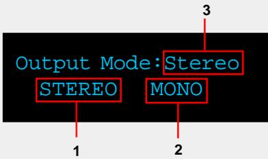
1 - STEREO mode produces 2 output signals. This is standard two channel stereo mode.
