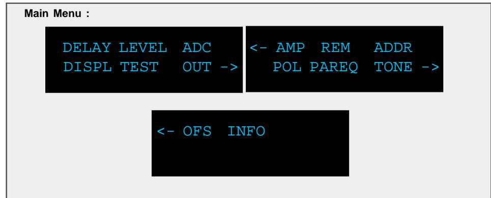
To enter the Menu selection pages press the “MENU” button. Use the “LEFT” and “RIGHT” navigational buttons to highlight an option with the selection cursor and to proceed to a new page. To enter a highlighted option press the “ENTER” button. Once you are in a menu option use the “MENU” button to go back one step (from sub-menus) with each press or to return to the main operating screen.
