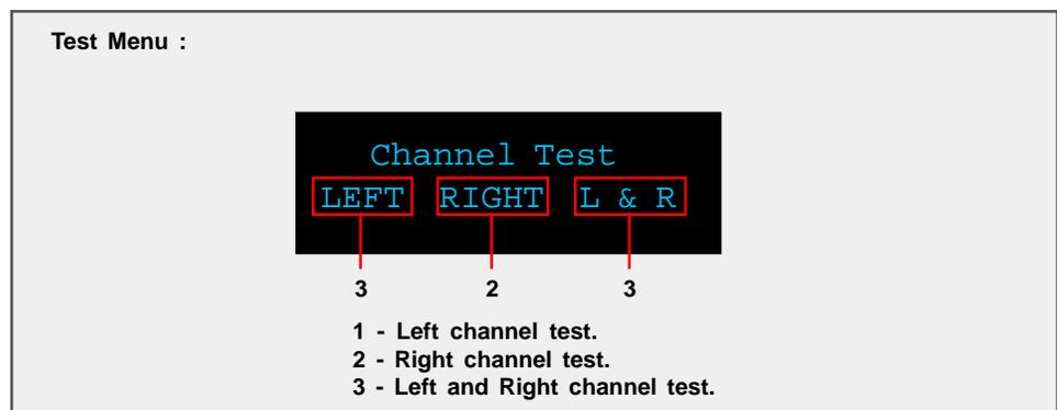
Use the “LEFT” and “RIGHT” buttons to highlight the desired option and select it by pressing the “ENTER” button. The pink noise will output from either the “LEFT”, “RIGHT”, or “L & R” channels combined while the “ENTER” button is pressed. The test tone will stop when the enter button is released.
