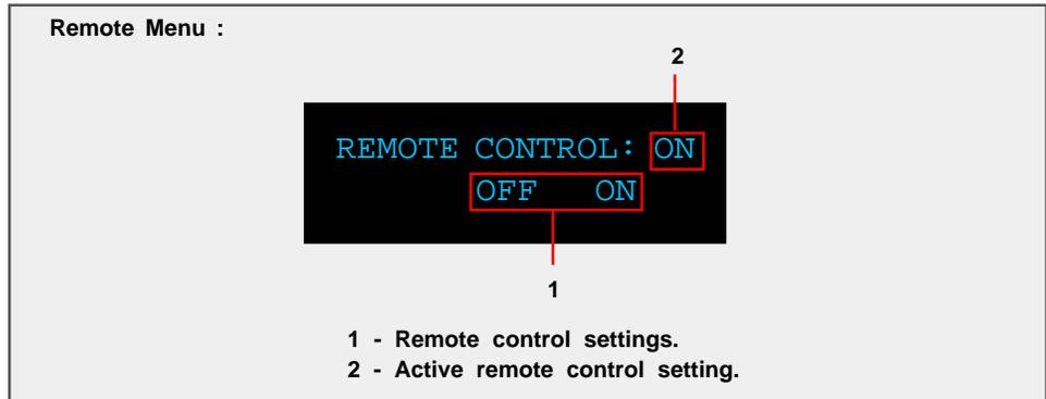
Use the “LEFT” and “RIGHT” buttons to highlight the desired option and select it with the “ENTER” button.
