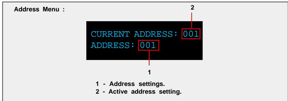
Use the “UP” and “DOWN” navigational buttons to select the desired system address and then press the “ENTER” button to select it.
