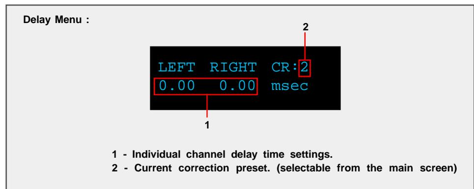
Use the “LEFT” and “RIGHT” navigational buttons to highlight an option and use the “UP” and “Down” buttons to change its value .
