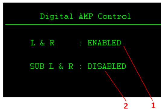
For example, one amplifier can be used for main left and right channel and second one can be used for the left and right subwoofer channels. If two TacT digital amplifiers are connected, both options (1) and (2) should be set to **ENABLED**. If one Tact digital amplifier is connected only one option should be set to **ENABLED** and the other one should be set to **DISABLED**. Enable should only be set for the output that uses Tact digital amplifiers.
