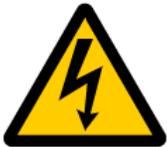
The lightning with arrowhead symbol within an equilateral triangle is intended to alert the user to the presence of "Dangerous Voltage" within the product's enclosure that maybe of sufficient magnitude to constitute a risk of electrical shock to a person.
